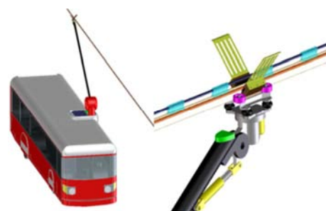
Figure 1. New concept trolleybus (left) with ACTCCS controlled pantograph-head and single overhead catenary with two wires separated by an insulation strip (right).
