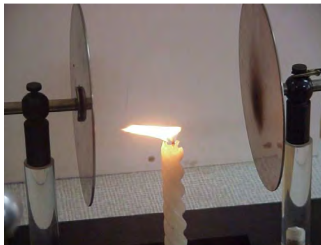
Figure 2. Candle flame under the influence of a left directed electric field: the upper part of the flame is directed to the left, and the lower part is directed to the right.
