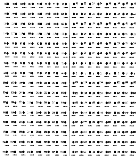
Fig. 2. Constellation diagram for 256-QAM [5].
