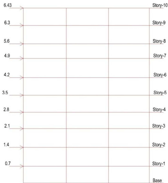
Figure 6. Elevation view of ten-storied building (point load applied on column line-4 in kips).
