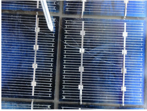
Figure 4. Cracked front glass of a solar module.
