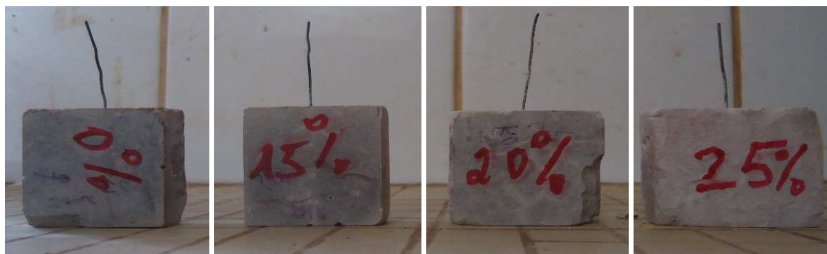
Figure 4. Images of specimens containing various proportions of RHA.
