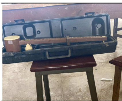
Figure 9. Mud balance used to determine mud density.
