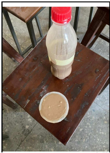
Figure 12. determination of mud cake thickness.
