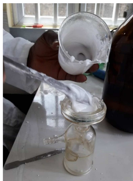
Figure 2. Casting on the composite membrane.
