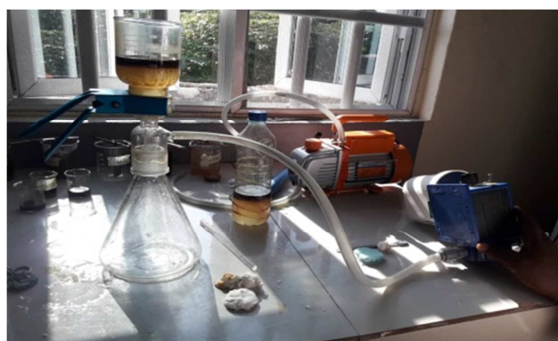
Figure 3. Membrane separation process using vacuum pump.
