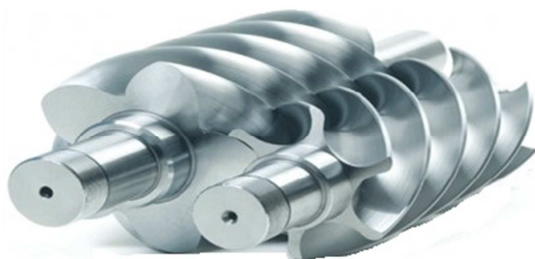
Figure 5. Rotor meshing of the screw expander.
