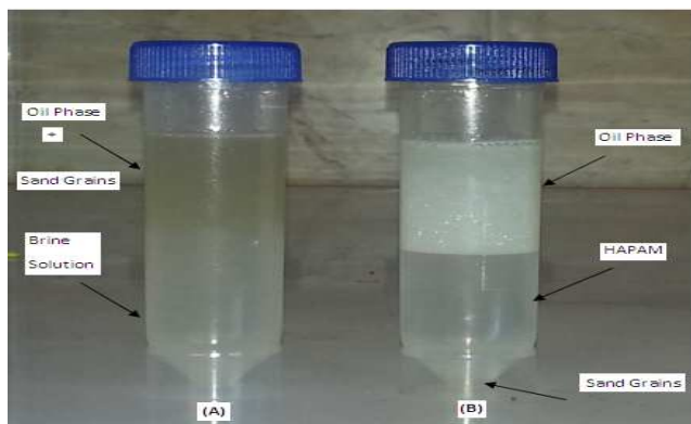
Fig. 17. Two-phase separation test.
