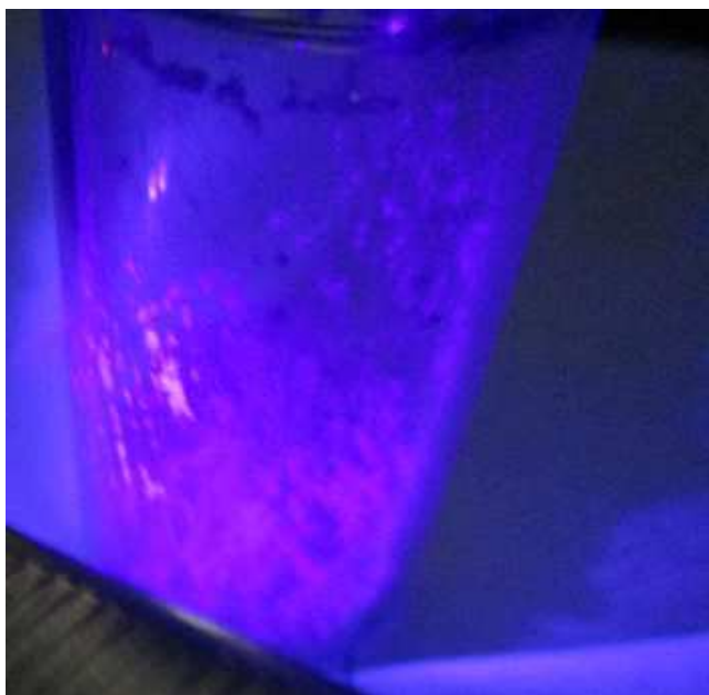
Fig. 5. Photo of PL from reduced Si nanoparticles.
