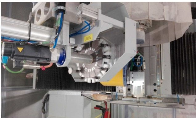
Figure 3. Main spindle and the tool storage with 12 tool places.
