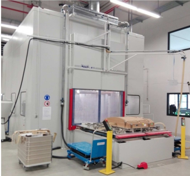
Figure 2. MAKa M7t type CNC driven milling machine [1].
