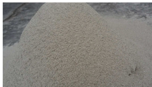
Figure 4. Construction debris after passing through 600 \mu m sieve.
