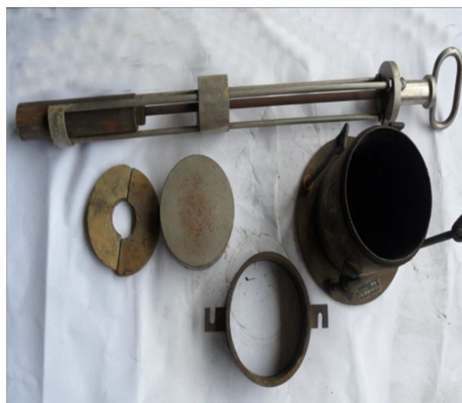
Figure 6. Compaction mould and rammer.
