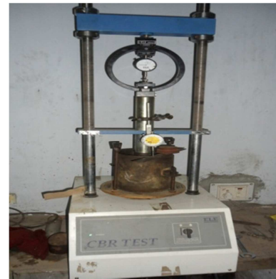
Figure 8. CBR testing apparatus.
