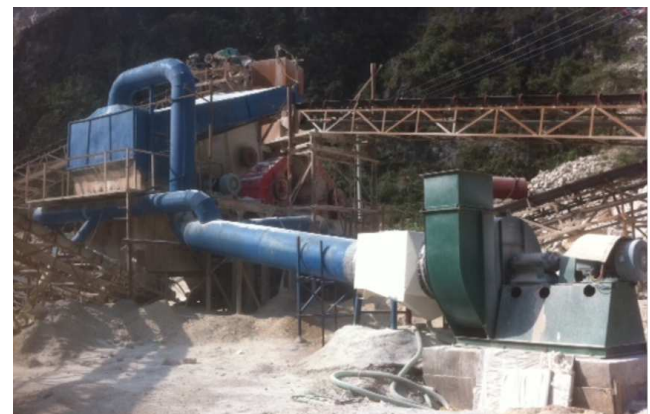
Figure 7. Closed dust extraction and purification system.
