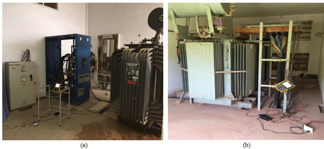
Figure 3. (a) Measurement Setup at the Auditorium Substation; (b) Measurement Setup at the Control Station.
