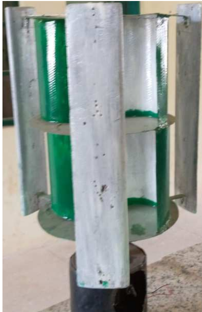
Figure 6. Lab scale hybrid VAWT showing various design components.
