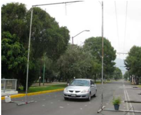
Figure 8. Vehicle under test crosses through the portal.
