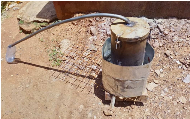
Figure 1. Complete assembly of the reactor and condensing system from the Nabisunsa stage welding station.
