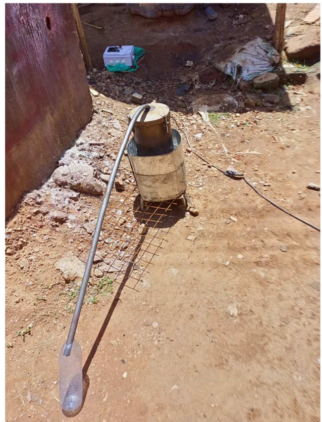
Figure 4. A complete setup of a pyrolysis reactor and a temperature-controlling system.
