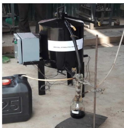
Figure 2. Pyrolyser Experimental Set-Up.
