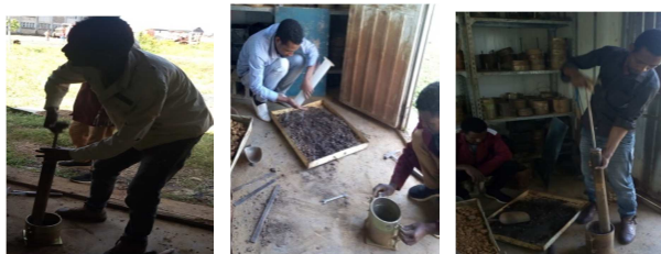
Figure 6. Proctor test (Photo taken by Kasahun 25/10/202).
