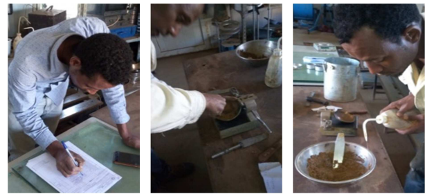
Figure 4. Atterberg's Limit (photo taken by Kasahun 10.10.2020@10:40AM).
