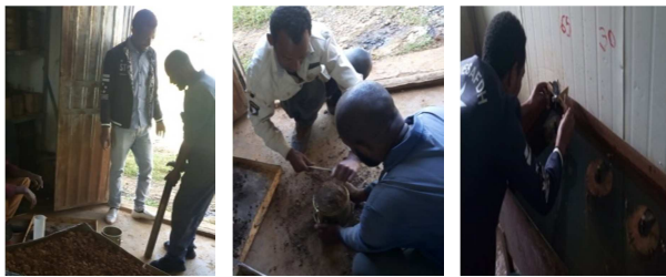
Figure 5. CBR test (photo taken by Imiru 17/10/2020@11:15 AM).
