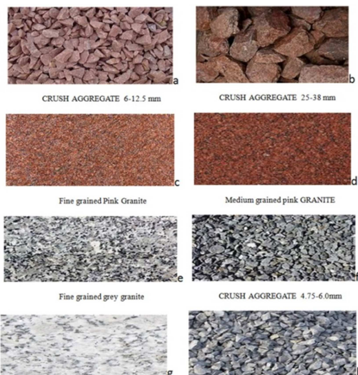
Figure 2. A GRANITE AGGREGATE SAMPLES (a, b, c, d, e, f, g, h).
