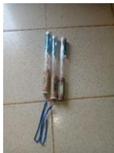
Figure 3. Digital thermometer with liquid immersion probe.
