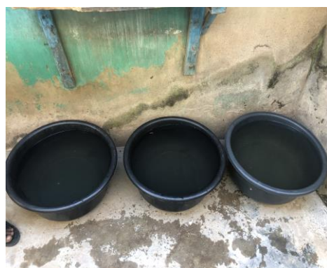
Figure 2. Primary Water Treatment (PWT) In the initial phase of water treatment, the polluted water was allowed to settle, facilitating the process of decantation.
