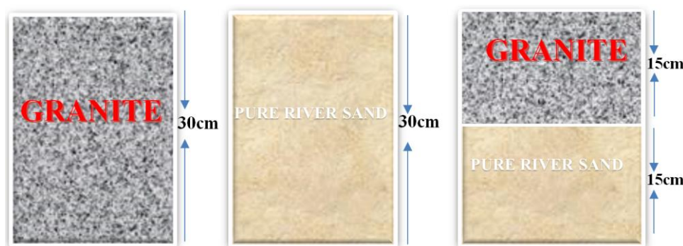
Figure 1. Arrangement of the filtration materials in the sole and combined filtration facility.
