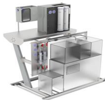
Figure 2. Schematic Diagram of the Pilot-Scale Ultrafiltration System.
