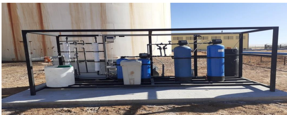
Figure 1. Integrated Membrane Process for EoR Application.
