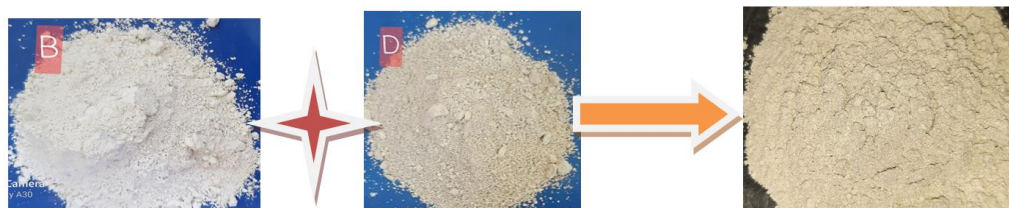
Figure 4. Kaolin powder plus limestone powder gives the normal raw material mixture.
