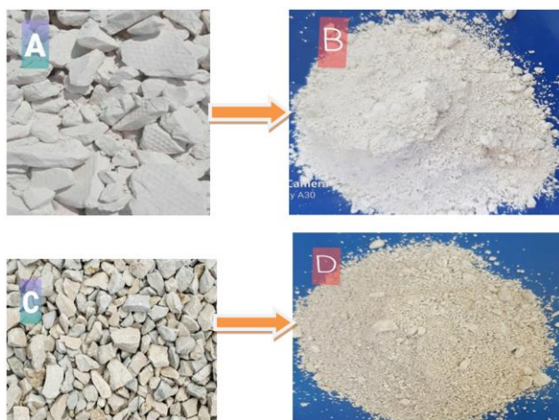
Figure 3. Raw Kaolin (A), Kaolin Powder (B), Raw Limestone (C) and Fine Limestone Powder (D).
