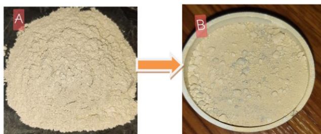
Figure 5. (A) Mixture of Geo Minerals and (B) Calcined Geo Mineral.
