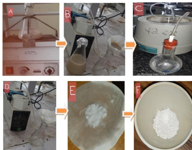
Figure 6. Leaching (A), 1 st Filtration (B), Carbonation (C), 2 nd Filtration (D), Aluminum Hydroxide (E) and Aluminum Oxide (F).
