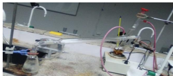
Figure 5. Transesterification experimental set up.
