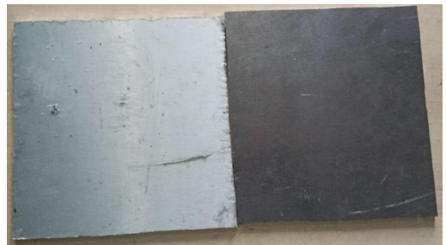
Figure 14. Aluminium 6061 sheet 50*50 mm with 5mm thickness.
