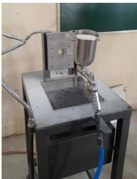
Figure 17. Erosion Testing setup.
