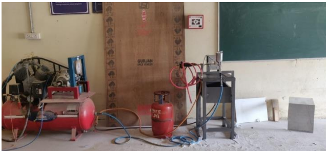
Figure 12. Fabricated Burner Rig.
