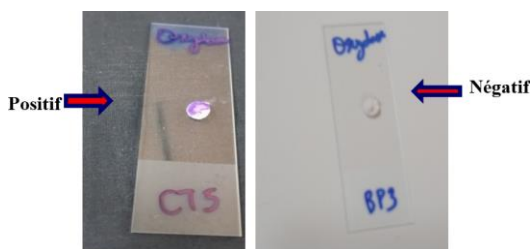
Figure 7. Positive and negative results of strains in the oxidase test.
