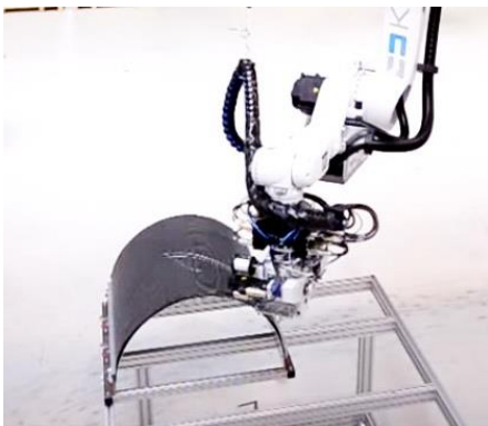
Figure 14. Application of 3D sewing technology on the outer and inner surface of a cylindrical part (Pfaff) [13].
