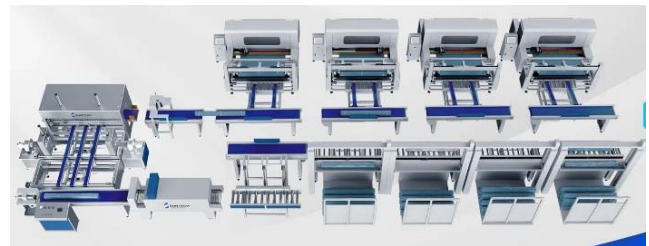
Figure 11. Roll wrapping robot, linked to a group of fabric inspection machines (Suntech).
