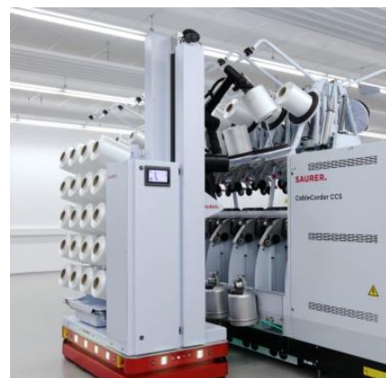
Figure 7. Saurer AGV robot for placing of cones.
