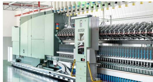
Figure 6. Rieter ROBOspin robot for repairing of yarn breakage.
