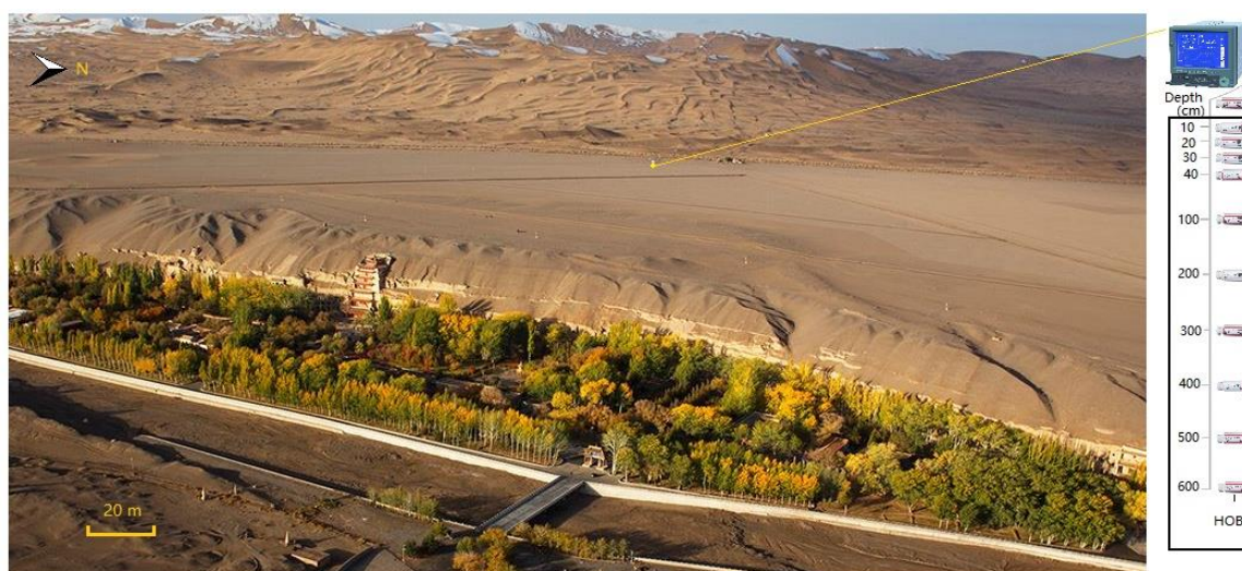
Figure 1. The location of the temperature monitoring experiments in the Gobi Desert region of the Dunhuang Mogao Grottoes. On the right is a schematic diagram showing the vertical arrangement of the buried temperature sensors.
