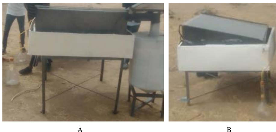
Figure 2. Snapshot of the Solar Stills (a) Modified Passive Still Distiller (b) Modified Convectional Still Distiller.
