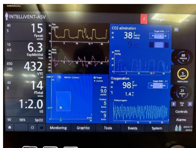
Figure 6. Visual interface of ventilator using ASV mode displaying CO 2 elimination and Oxygenation with real-time EtCO 2 and SpO 2 within target range.
