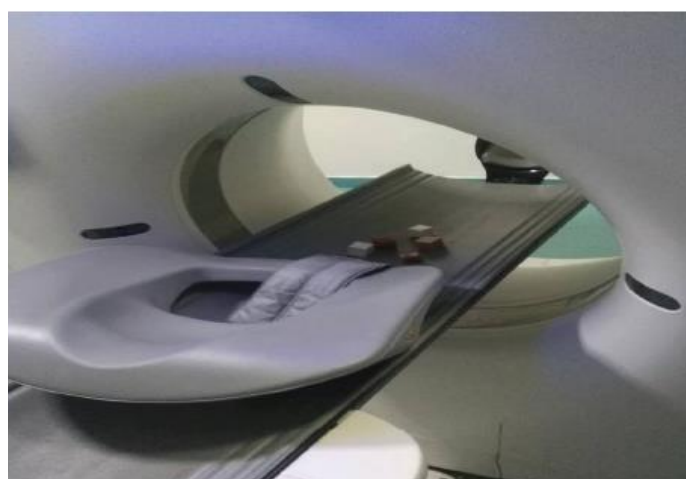
Figure 1. Image of the samples during measurements of HU using CT scanner.
