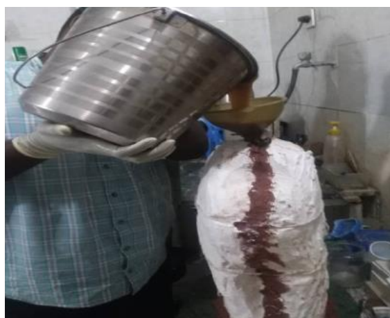
(i) pouring of mixed soft tissue equivalent materials inside the mold.
