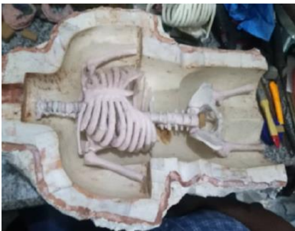
(g) inserting and fixing the skeletal and lung inside the mold.
