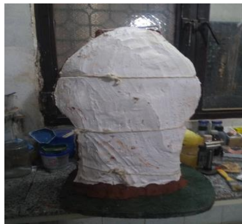
(h) preparing the external mold before pour the mixer inside the mold.
