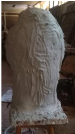
(e) covering the body with gypsum to give the external mold of trunk.
