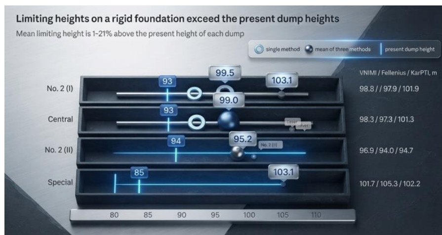
Figure 1. Limiting stable height of the Kalmakir dumps on a rigid foundation by three methods, compared with the present dump height.
