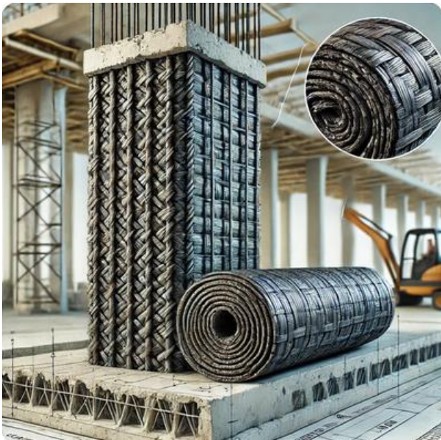
Figure 11. Fiber-reinforced polymer (FRP) used for reinforcing concrete columns.
