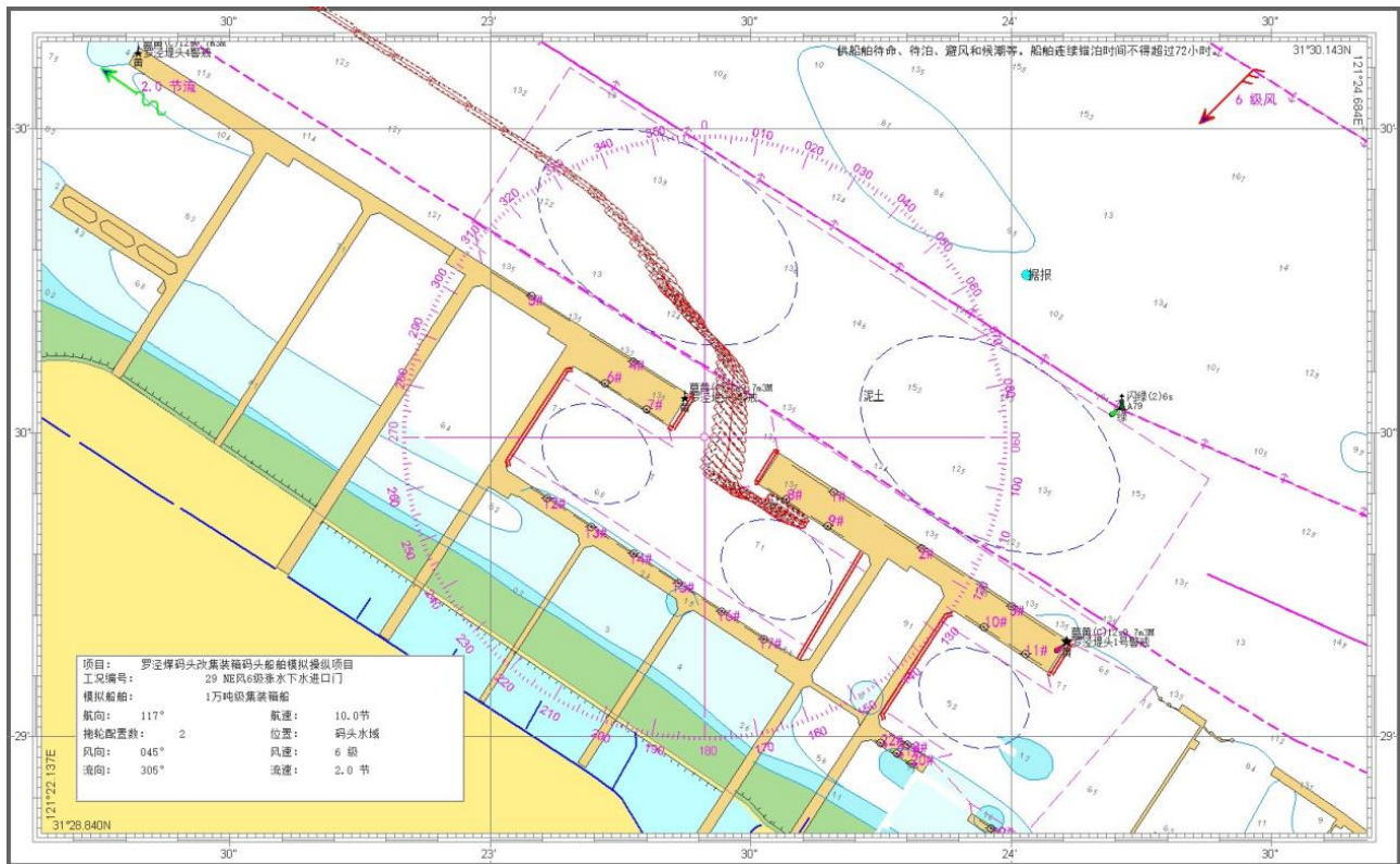
Figure 9. Track diagram of the 10,000-ton container ship NE Class 6 (inlet gate).
