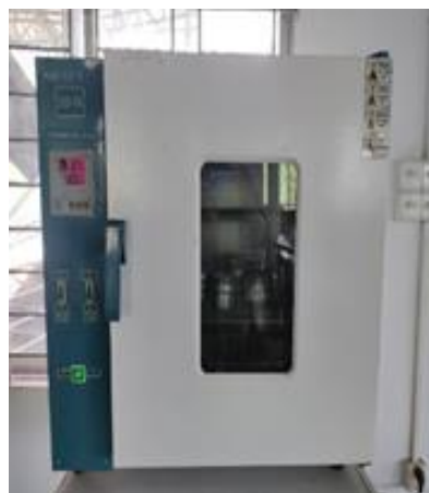
Figure 1. Oven dry for Moisture Content.
