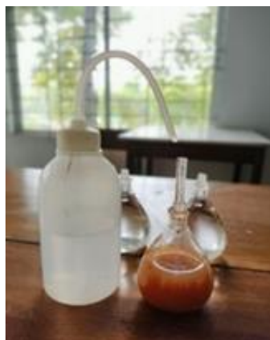
Figure 2. Specific Gravity Determination.
