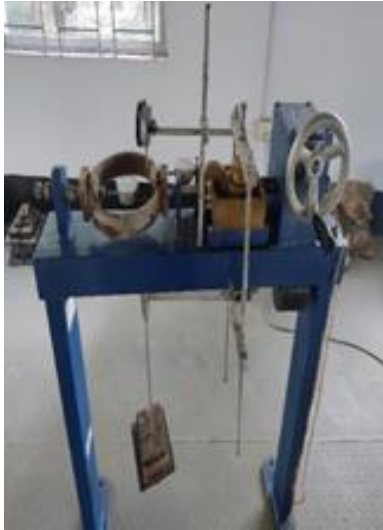
Figure 4. Direct Shear Test.
