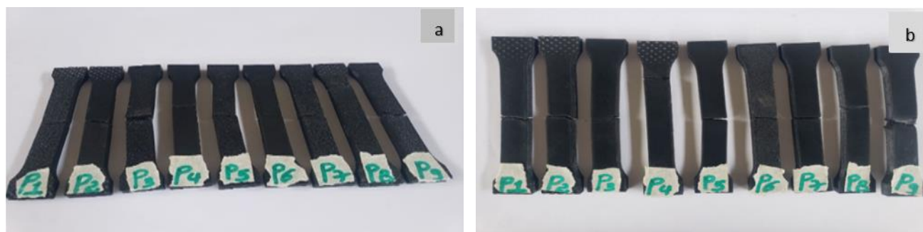
Figure 10. Result of fracture for PETG specimen after tensile and compression test.
