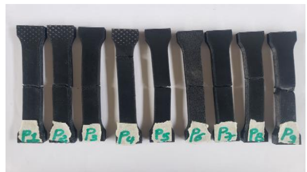
Figure 9. PETG fractured samples after compression test.
