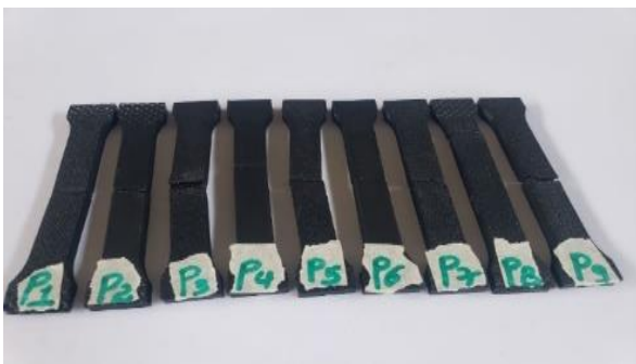
Figure 7. PETG fractured samples after tensile test.
