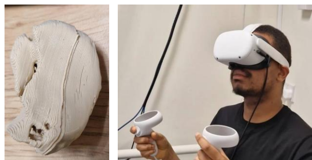
Figure 4. Left: physical 3D-printed glenoid model produced via the institutional workflow. Right: corresponding VR environment (Unity) rendering of the same segmented anatomy, viewed via head-mounted display.
