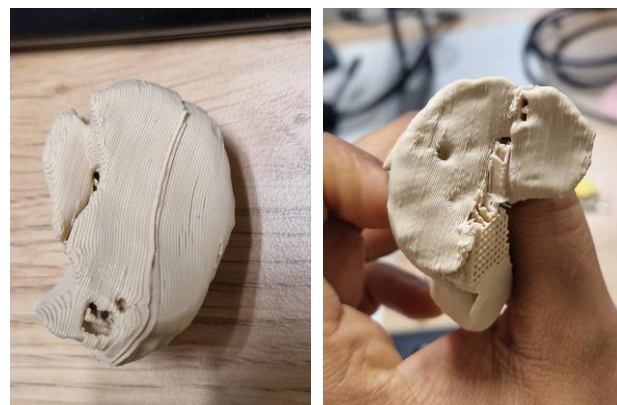
Figure 5. Left: external surface detail of the printed glenoid segment, showing visible FDM layer lines and a fracture/seam line at the Meshmixer sectioning plane. Right: cross-sectional view of a fractured print, showing internal lattice infill and structural failure at a thin, comminuted region.
