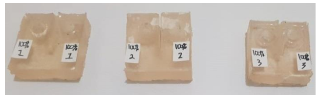
Figure 5. Crack Test Specimen.
