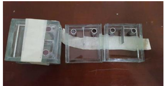
Figure 4. Crack test Specimen mold.
