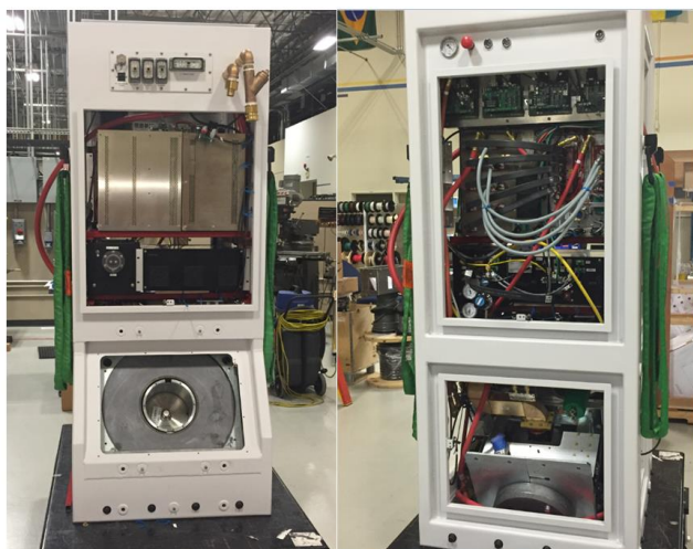
Figure 34. A single block, SSM based Mi6SSM (Tower) LINAC system primarily used for Security Screening. Temperature-Regulated Water Chiller and Operator Console come separately and not shown.
