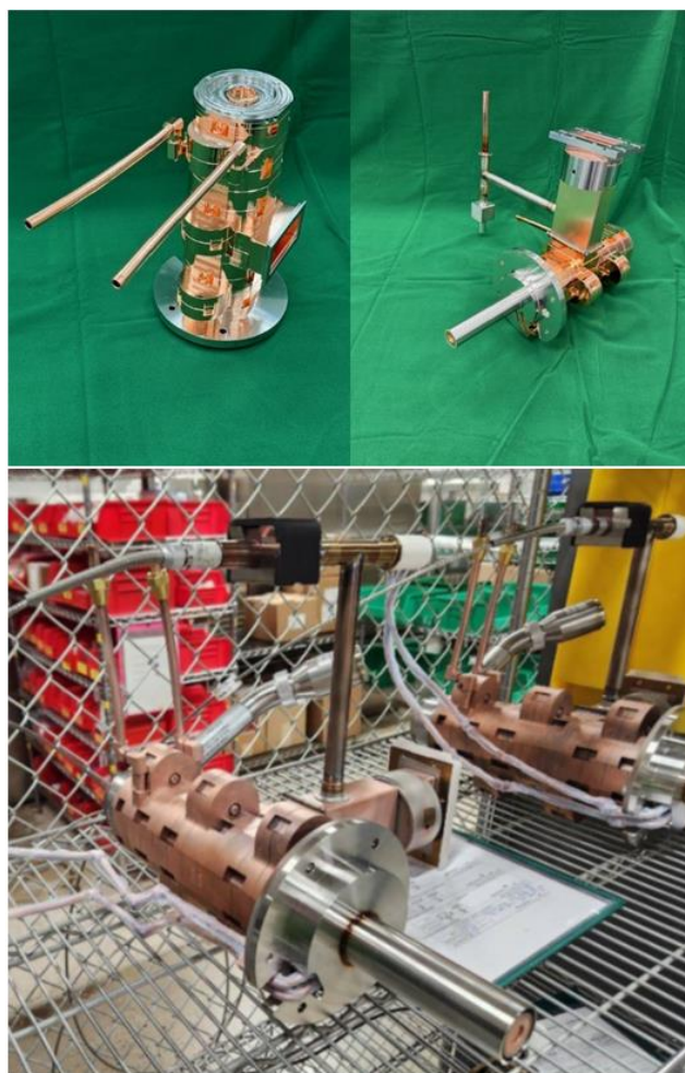
Figure 15. ABC-6-S-M-X In order as shown: Final Brazed Assembly (1) Vacuum Assembly ready for vacuum processing (2); Completed, ready to ship ABC-6-S-M-X-D (3).
