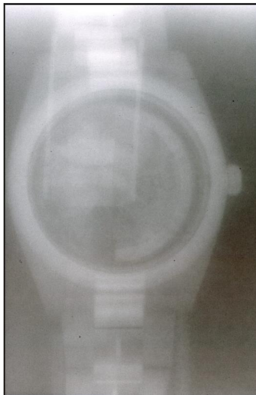
Figure 30. A film image of a watch with a metal wrist band behind one-inch-thick steel plate. One can clearly see a thin plate of watch band behind the watch.
