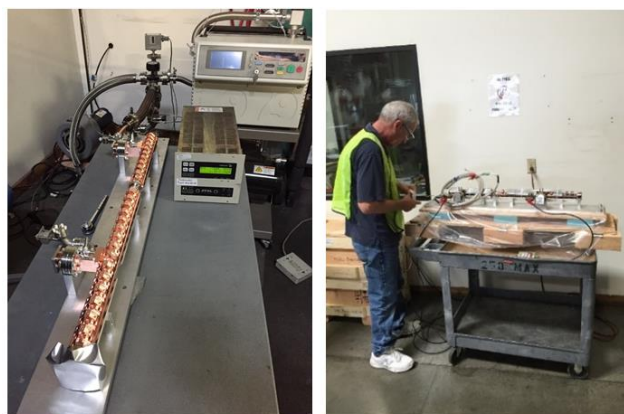
Figure 3. 12 MeV electron beam X-Band ABC equipped with a triode electron gun (ABC-12ER-X-E-T).
