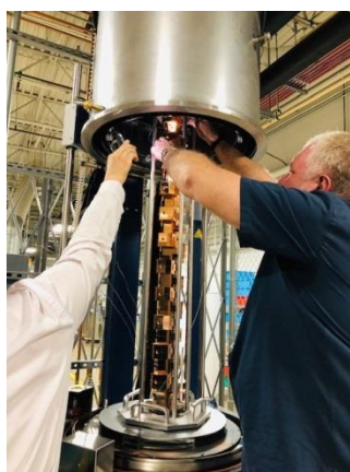
Figure 19. ABC-9-S-O-X-T being set in a brazing furnace.
