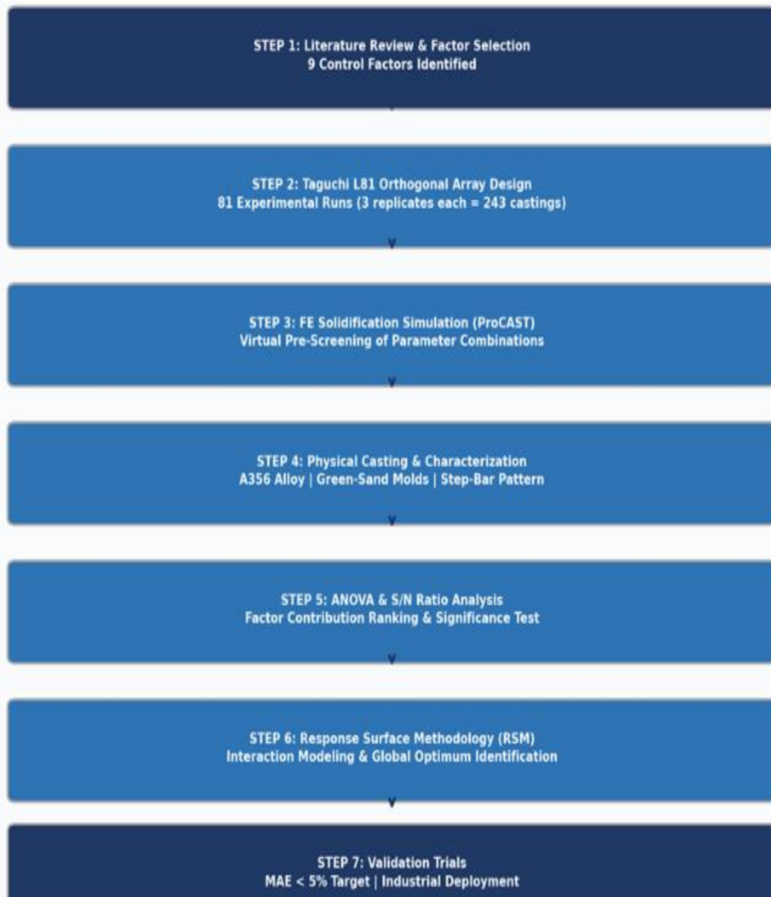
Figure 1. Multi-Parameter Optimization Framework (MPOF) - seven-step methodology flowchart showing the integration of Taguchi DOE, FE simulation, and RSM.
