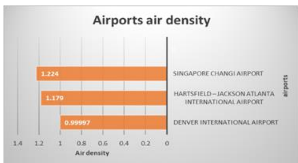
Figure 4. Air density at different elevations.
