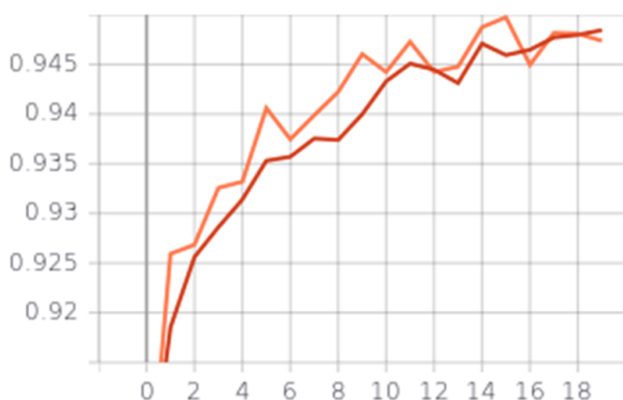
Figure 3. Validation accuracy over 20 epochs for model 1. Weighted CE in orange, Dice Loss in red.
