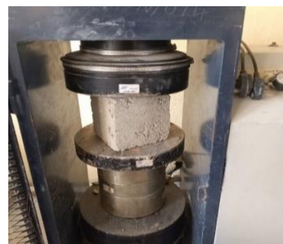
Figure 11. Compressive strength test.
