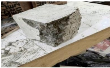
Figure 13. Crushed GC2 granite concrete.
