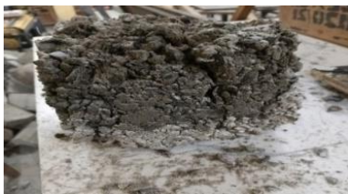
Figure 14. Crushed PKS concrete.
