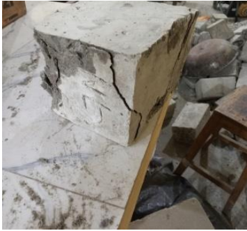
Figure 12. Crushed GC1 granite concrete.
