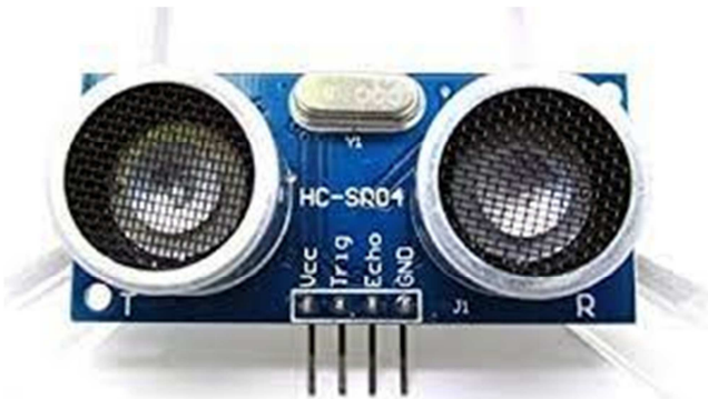
Figure 2. Ultrasonic Sensor HC-SR04.
