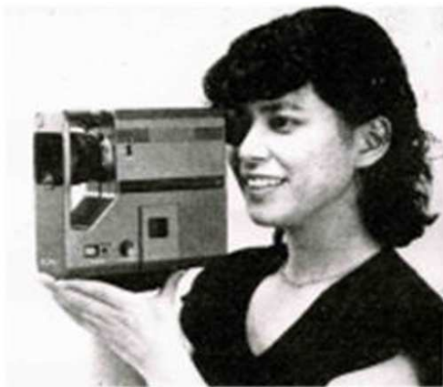
Sony 1980 Video Movie has in one body an 8 mm VTR and One Chip FT CCD Image Sensor with the PNP Double Junction type Pinned Photodiode developed by Hagiwara in 1978
