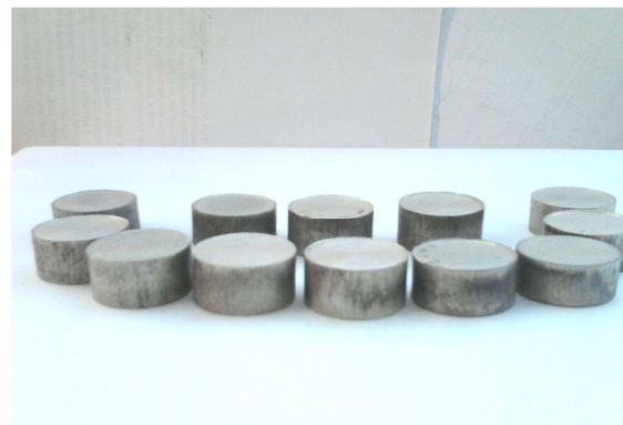
Figure 12. Sintered Specimen for Various Sample Pieces (front orientation).
