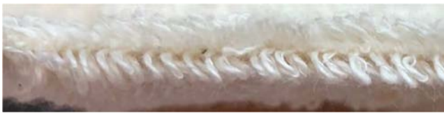
(c) cross section picture of terry fabric sample [21].
