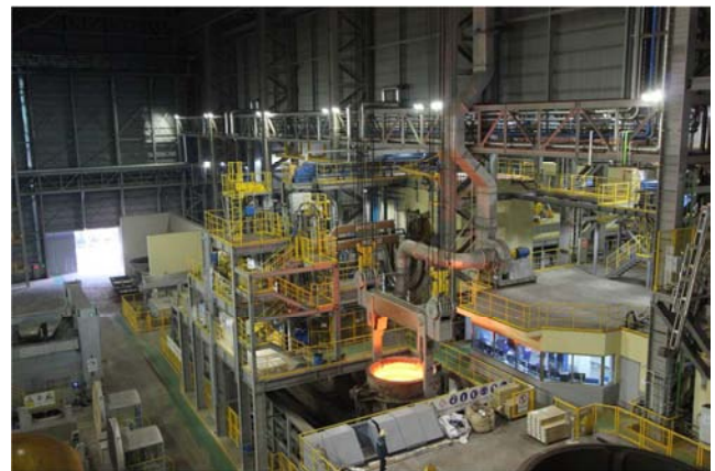
Figure 3. Ladle Furnace.
