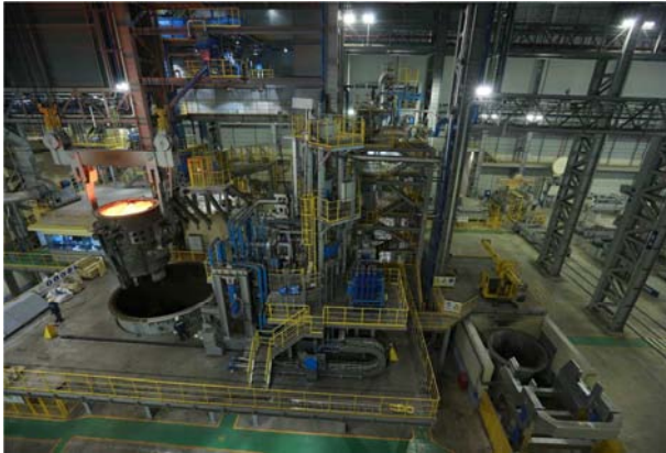
Figure 4. Vacuum Degassing / Vacuum Oxygen Decarburization.
