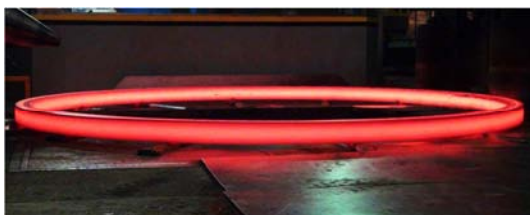
Figure 11. Ring rolled product manufactured with \varnothing 1,000 round bloom.
